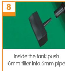
Inside the tank push 6mm filter into 6mm pipe
